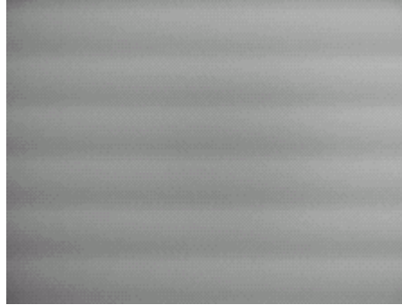
Figure 35: Flicker in image of white uniform object illuminated by strong fluorescent light
